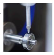
AST's in-house capabilities, including a clean room, proved critical to the project's success. The ability to disassemble the bearings, replace the steel balls with ceramic balls, re-install the retainer, and perform final inspection in a cleanroom environment made the entire process turn-key for the manufacturer, a rarity in the bearings industry.
