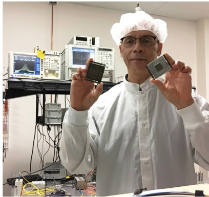
Brice holding up one of his innovations – integration of optical waveguides into large ASIC chip substrate.
